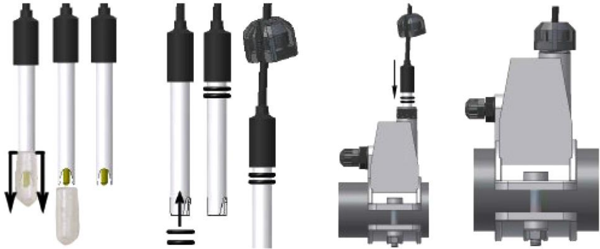
Fig. 3 – Mounting the probe in the probe-holder
