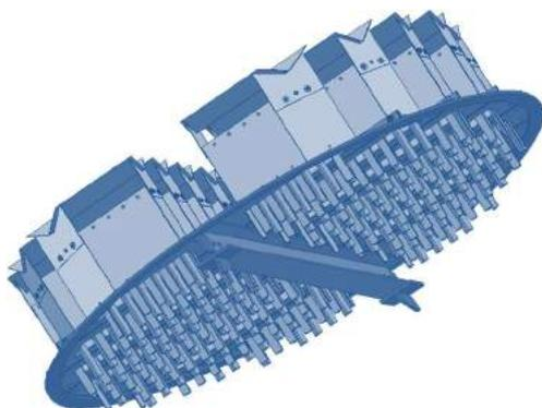
A mixed feed that flashes when it enters the column between beds can lead to maldistribution. In this instance, there may be a requirement for a complex inlet distributor design that produces both, an even composition and flow rate at each point in the column cross section.
