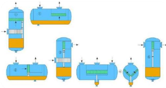
As the hydrocarbon gas/oil/water mixture is extracted from below the sea bed, the mixture is fed into a production separator vessel on the offshore platform.
