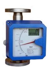
Series LZ variable-area flow-meter by float position and according to fluid dynamics and magnetic coupling system. Adopts rugged, all-metal construction and HART communication and especially foe indicatory the instantaneous flow value of liquids , gases and vapor.
