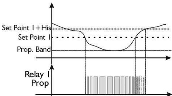
(\* when equal times are set for ON Timer and OFF Timer, the instrument calculates a total period that it automatically modifies in relation to the chemical measurement's variation. In the hysteresis band, it doses at the minimum value)
