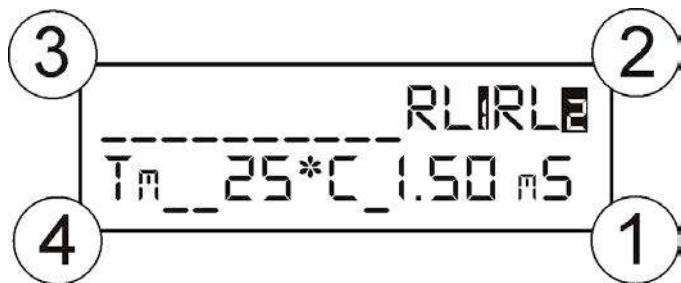
Area 1 = Display of chemical conductivity measurement
