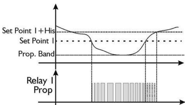
(\* when equal times are set for ON Timer and OFF Timer, the instrument calculates a total period that it automatically modifies in relation to the chemical measurement's variation. In the hysteresis band, it doses at the minimum value)
