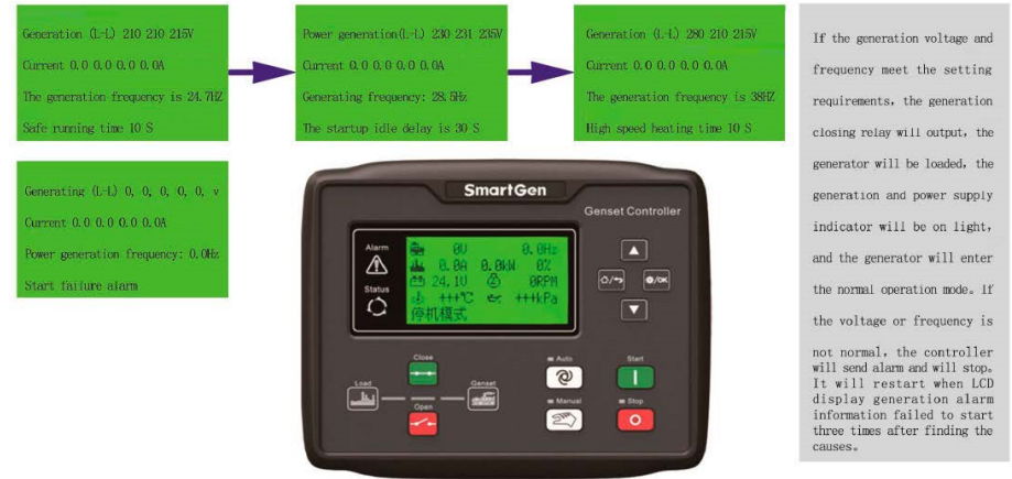
Normal operation of generator
